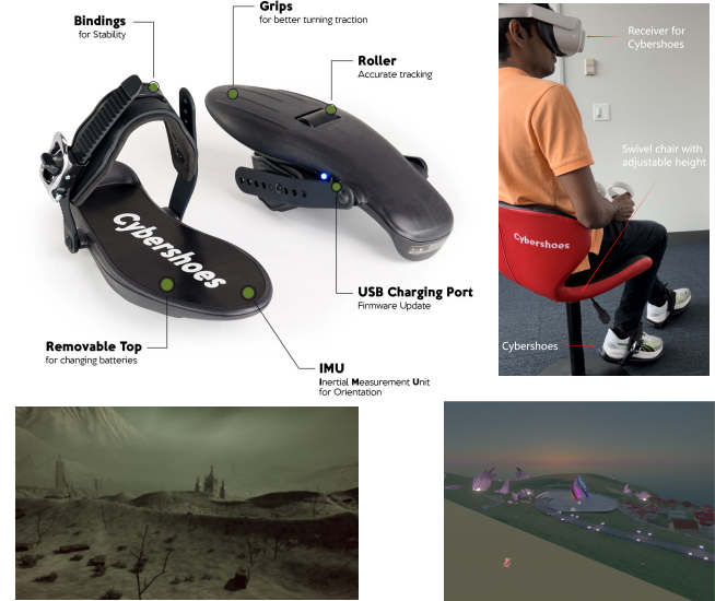
Figure 1: (Top-Left) Components of the Cybershoes (image from https://www.cybershoes.com/ ). (Top-Right) A participant wearing Cybershoes while navigating VR worlds for sightseeing tasks. Scenes from two VR worlds: (Bottom-Left) Eternal Ash [2] and (Bottom-Right) Eventide [3].
