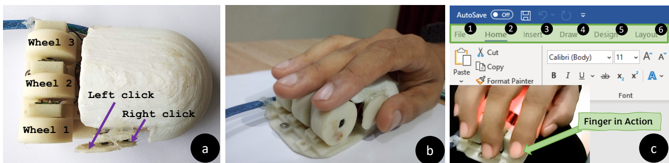
Figure 1: WHEELER input device and its usage in the wild. (a) shows a 3D-printed implementation of Wheeler having three wheels and two push buttons (primary and secondary) on the side; (b) shows a blind user holding the device, placing three central fingers on the three wheels, and the thumb over the two side buttons; (c) shows how a blind user can navigate the multi-level, hierarchical menu (e.g., Microsoft Word's ribbon menu) using Wheeler's H-nav mode. The pale green rectangle at the top shows the first level menu in the app, with the numbers 1-6 each representing individual menu items (e.g., File, Home, Insert). The user is using Wheel 1 with their index finger . By rotating the wheel, the user can move the focus in the menu. The other two wheels are used for navigating the second ((e.g., Font) and third-level menu items (e.g., Boldface, Italic).
